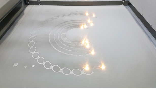
Fig. 4 Active laser exposure of metal powder within the NXG 600E machine process chamber
