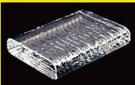
Nikon's i-line glass with high transmittance at the i-line wavelength
