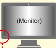
Backlight leakage from the edge causes brightness irregularity
